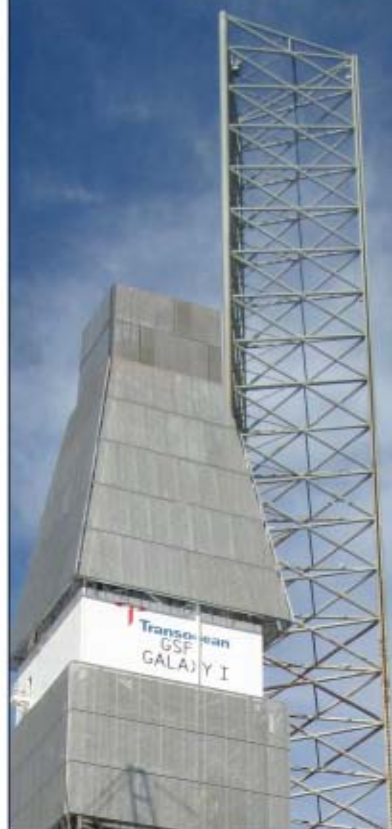
Heat Shield installation on the Galaxy 1
